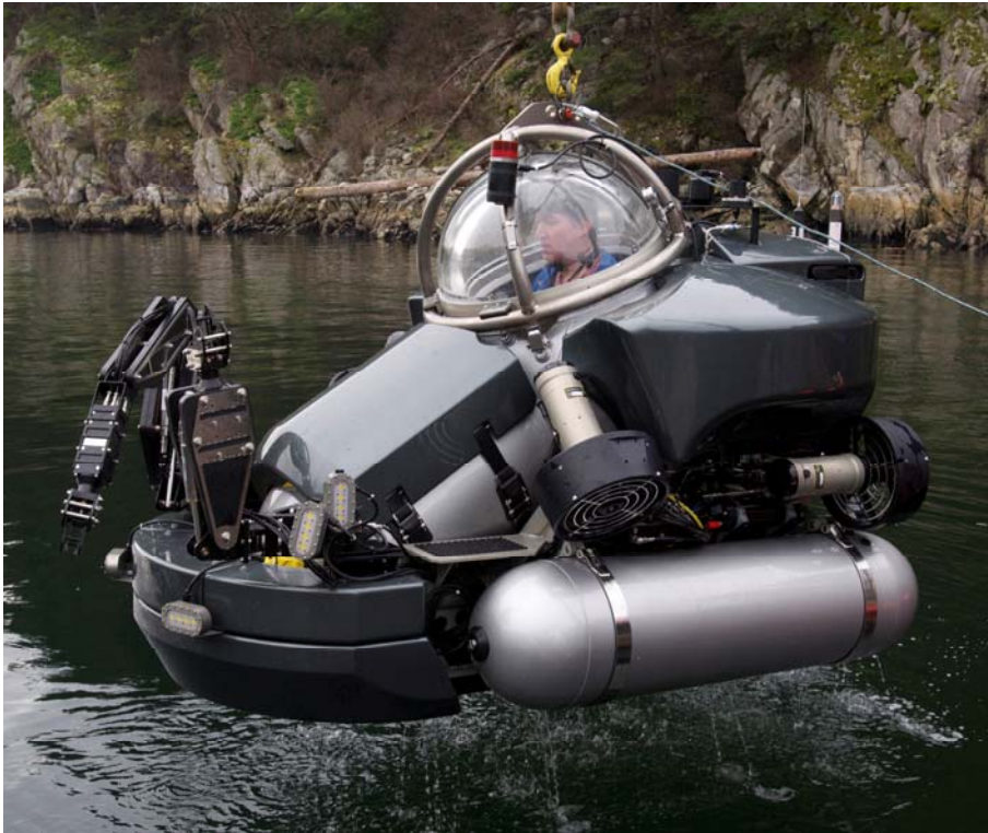
Nuytco's Single Deepworker manned submersible with Hydro-Lek CRA6 and RHD4 arms
