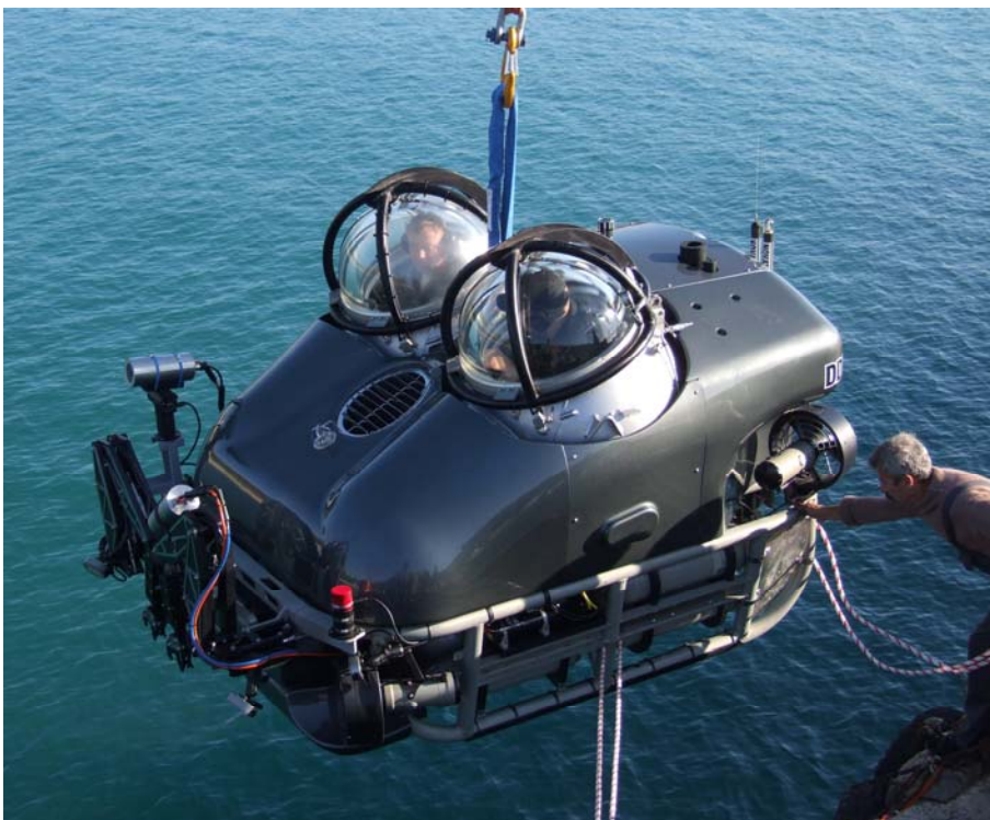
Nuytco's Dual Deepwater submersible with 2 Hydro-Lek CRA6 arms
