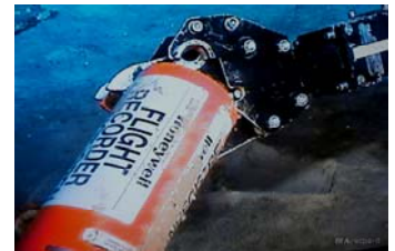
Hydro-Lek Manipulator recovering FDR box belonging to Air France Flight 447.
