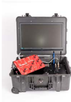
Figure 9: Hydro-Lek's Portable Surface Control Console for HyBIS
