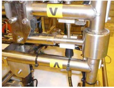
Detail showing the hydraulic release mechanism for various tool modules
