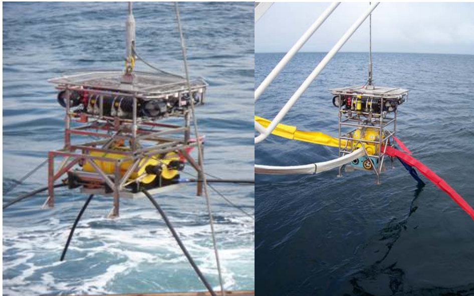
HyBIS with OBS deployment module for Geomar (left) and NOC (right)
