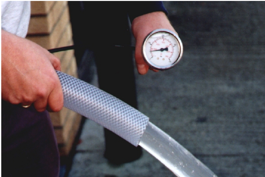
High pressure water entering the suction jet viewed from the suction end
